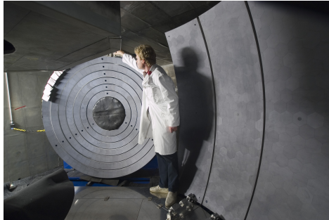
Fig. 3: The analyzers of SPHERES are made of the same Si(111) as the monochromator. For small scattering angles, they are shaped as rings; for large scattering angles, they are approximately rectangular sections of a sphere.
