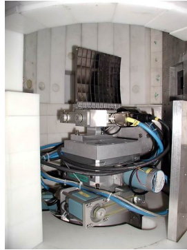
(b) PG-analyzer in the (opened) analyzer box. The horizontal curvature is changed by rotating the individual segments.
