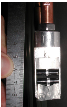
(e) Typical sample mounting for use of cryostat.
