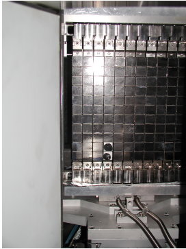
(a) Side view into the (opened) Monochromator shielding onto the PG-monochromator.
