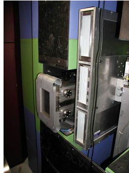
(d) Soller collimators in the automatic changer for \alpha_1 (in the primary beam.)
