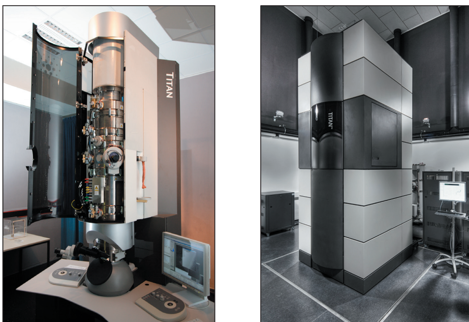
Fig. 1: (Left) FEI Titan 80-300 and (right) FEI Titan G3 50-300 PICO field emission transmission electron microscopes at Forschungszentrum Jülich. The instrument on the left is equipped with a spherical aberration corrector on the objective lens and has an information limit of 0.08 nm. Photograph courtesy of Ralf-Uwe Limbach (Forschungszentrum Jülich). The instrument on the right is a fourth generation transmission electron microscope equipped with a monochromator, a spherical aberration corrector on the condenser lens and a combined spherical and chromatic aberration corrector on the objective lens. It has an information limit for coherent high-resolution TEM of below 50 pm at 200 kV. Photograph courtesy of Christian Lünig ( www.arbeitsblende.de ).
