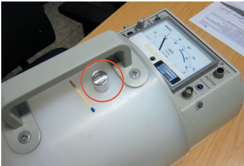
Fig. 1: AmBe neutron source used for detector calibration. The source's \alpha activity is 350 MBq, yielding a neutron production of 20000 n/s. The measured dose rate emitted by this source is about 10 \mu\text{Sv/h}
