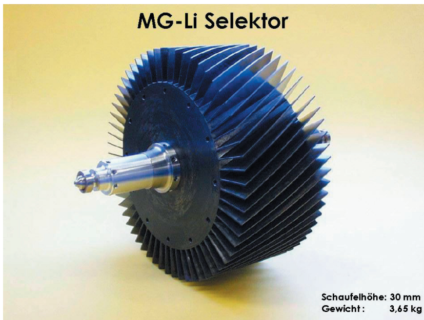
Fig. 5: Turbine wheel of the velocity selector used at KWS-3. The selector blades consist of a MgLi alloy with neutron absorbing ^6\text{Li} .
