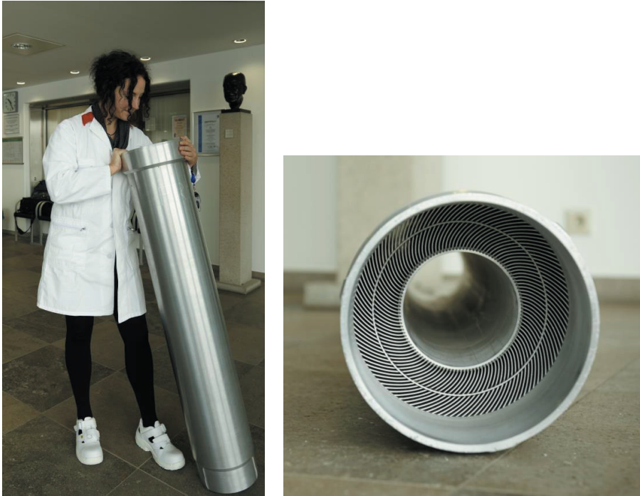
Fig. 4: A model of the fuel element of the FRM II research reactor. The inclined plates contain the fuel, the cooling water flows in between the fuel plates. The central channel is the position of the control rod. The core of FRM-2 is the most compact ^{235}\text{U} reactor core ever built.
