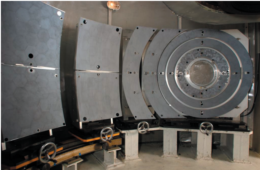
Fig. 12: Energy analyser bank of the backscattering spectrometer at FRJ-2. Every analyser section is a part of a sphere and is covered with perfectly aligned Si single crystals.
