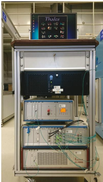
**Figure 3.3:** The Zahner EIS system (From up to down: PP211, IM6 and EL1000).
