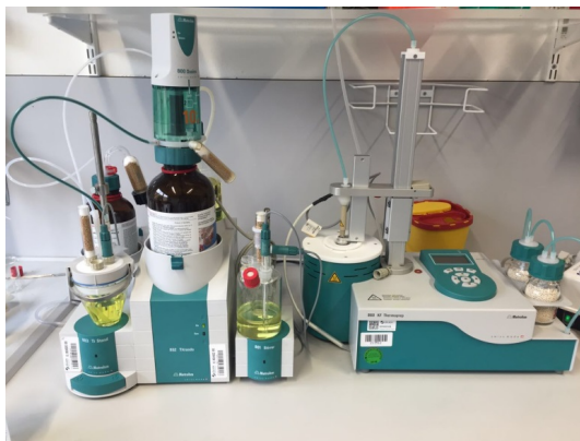
Figure 2.3: Karl Fischer Titration system
