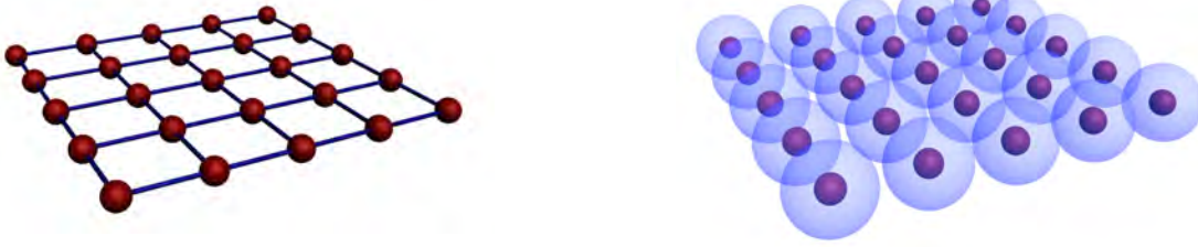
Fig. 1: Left: Illustration of the Hubbard model showing lattice sites on which electrons interact with Hubbard interaction U (red) connected by bonds through the hopping integrals t . Right: DMFT picture of model showing a collection of decoupled sites exerted to an electronic bath, as indicated by the blue spheres.
