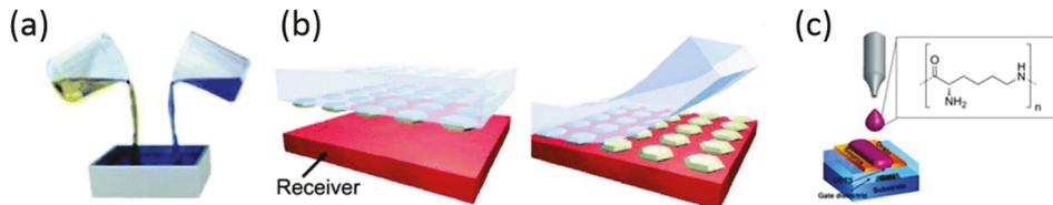
Figure 4. Various techniques for the deposition of molecules: (a) solution casting, (b) stamp printing, and (c) inkjet printing.
