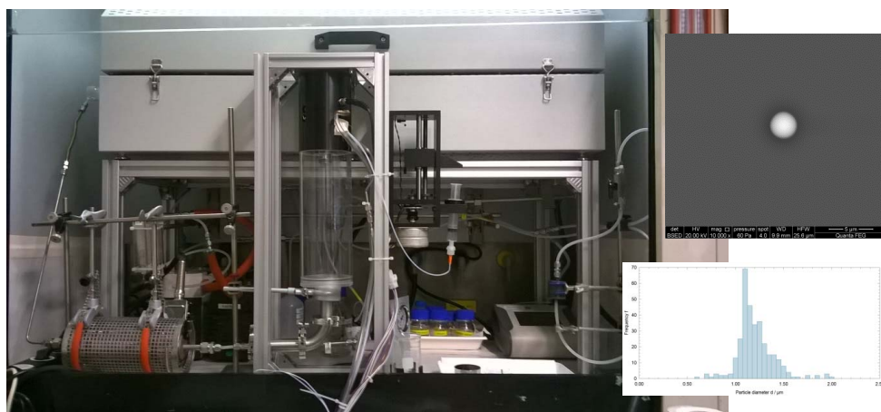
Fig. 15: Microparticle generator (left) and SEM micrograph of single particle (right-top) with particle size distribution (right-bottom).
