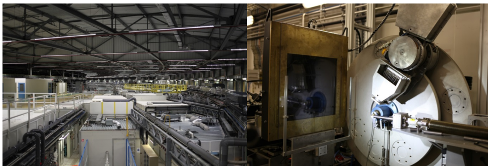
Fig. 6: Top view of the large experimental hall at the ESRF/Grenoble (left picture), and experimental setup of powder diffraction experiments on geopolymers using a 2D-detector at beamline ID22 at the ESRF (right picture).
