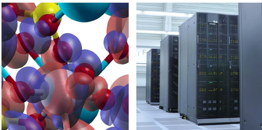
Fig. 5: Left: one of the electronic orbitals responsible for bonding between U atom (grey) and neighboring O atoms (red) in \text{Ba}_2(\text{UO}_2)_3(\text{PO}_4)_2 borophosphate. Interaction between Uranium f orbital and Oxygen p orbitals is clearly visible. An atomic scale analysis of charge distribution provides information on the bonding environment. Right: Computer cluster at RWTH Aachen used in the investigation within Jülich-Aachen research alliance (JARA-HPC).
