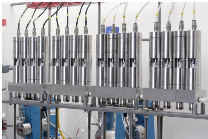
Fig. 9: Centrifugal contactors installed in the fume hood of IEK-6 laboratory
