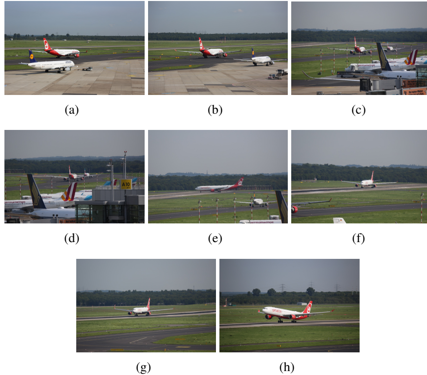
Figure 5 Collecting data through visual observation. The times of passing the checkpoints are noted and taxiing times between the checkpoints are calculated. (source: own pictures)
