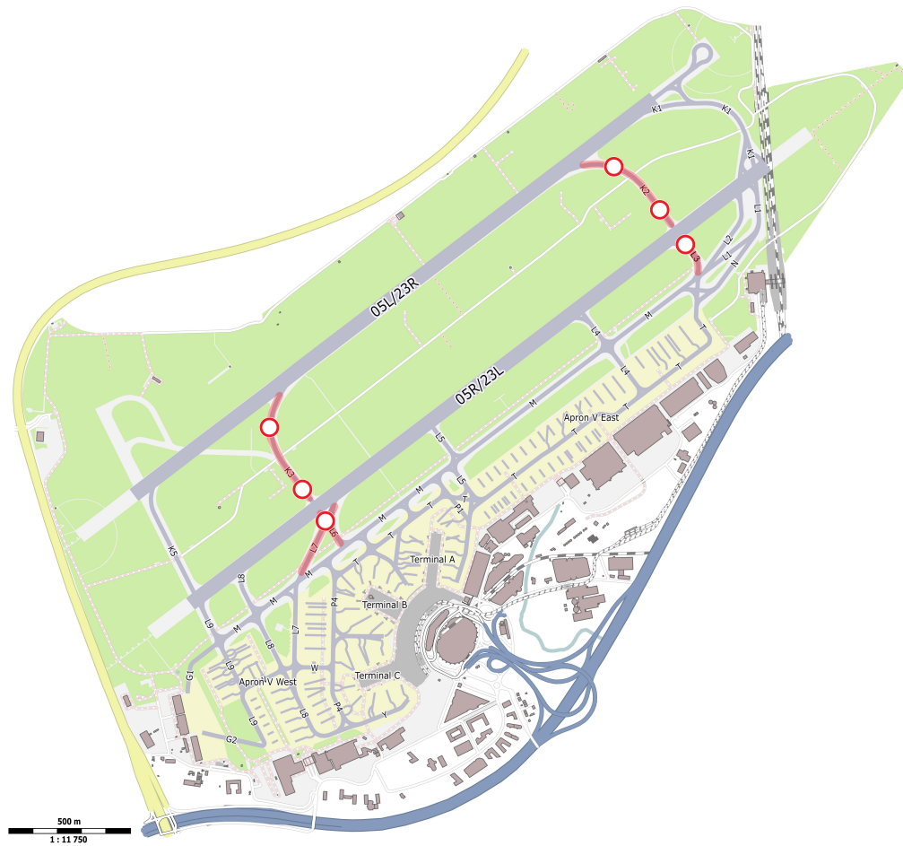
Figure 8 Closure of runway exits K2 and L3 (relevant if runway 05 is in use), as well as runway exits L3 and L6/L7 (relevant if runway 23 is in use). (Source: OpenStreetMap contributors (Licence ODbL) [22])
