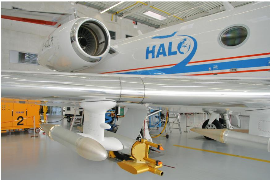
**Figure 2.2:** NIXE-CAPS mounted on HALO.
