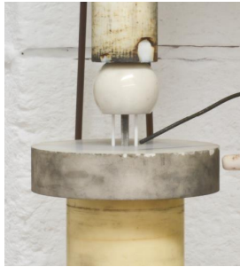
Figure 4-5: Compressive creep test set-up.
