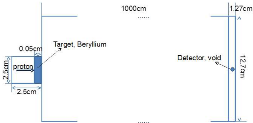
Fig. A1.1. MCNP model of the experimental arrangement described in [23] to measure neutron energy spectra from the ^9\text{Be}(p,n) reaction
