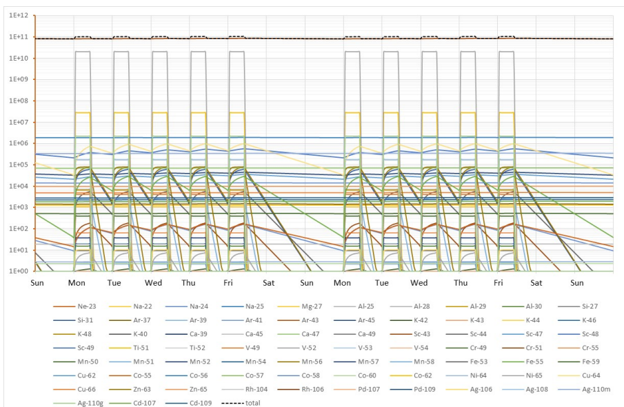
Fig. A6.4. Activity of the radionuclides formed by proton and neutron activation in the vanadium target ( m = 61.4 g) at week 39 and 40 out of 40 weeks of irradiation with 10 h of irradiation per working day and 5 working days per week (in total 2000 h of irradiation)
