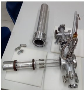
Fig. 3.18. Cold moderator vessel with cryogenic supply and monitoring (left). Technical drawing of the moderator vessel (left). The total length of the vessel is 600 mm.
