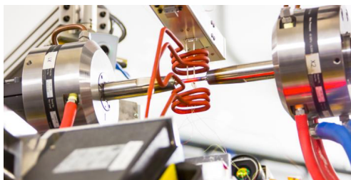
Fig. 2.3. Studying nickel-based superalloys with neutron diffraction [10]
