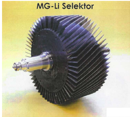
Fig. 5.2: The neutron velocity selector of the small angle scattering instrument KWS-3 at the research reactor Garching FRM-2. This selector was especially manufactured for larger wavelengths (above 7\text{\AA} ).
