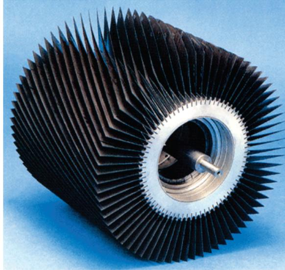
**Fig. 1:** Rotor of a mechanical neutron velocity selector. The blades are coated with neutron absorbing material. In SPHERES, such a selector is used as a pre-monochromator that reduces the incoming white spectrum to about 0.7%. © Astrium GmbH.
