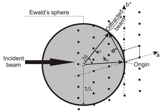
Figure 3: Illustration of diffraction using the Ewald's sphere.
