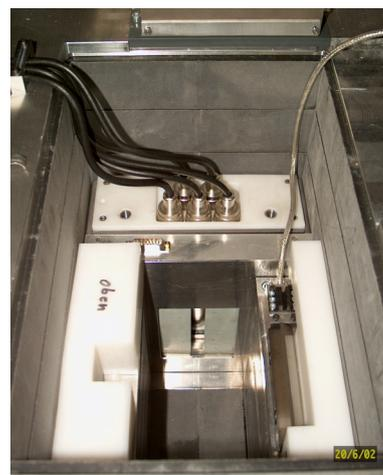
f) Detector, consists of 5  $^3\text{He}$  tubes**Fig 5** Elements of PUMA
