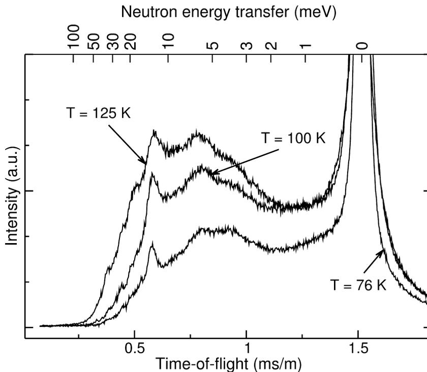
**Fig. 1:** Neutron time-of-flight spectrum of pentafluorotoluene, taken from [3]. Elastic scattering happens at energy transfer zero, quasielastic scattering in a region of approximately  $0 \pm 1$  meV, inelastic scattering at larger energy transfers.
