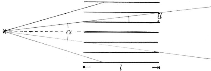
**Figure 9:** Drawing of a Soller collimator. The divergence of the outgoing beam is  $\tan(\alpha/2) = d/l$ , which is in the example ca.  $18^\circ$ . On PANDA the collimation can be chosen between 15 and 80 minutes.
