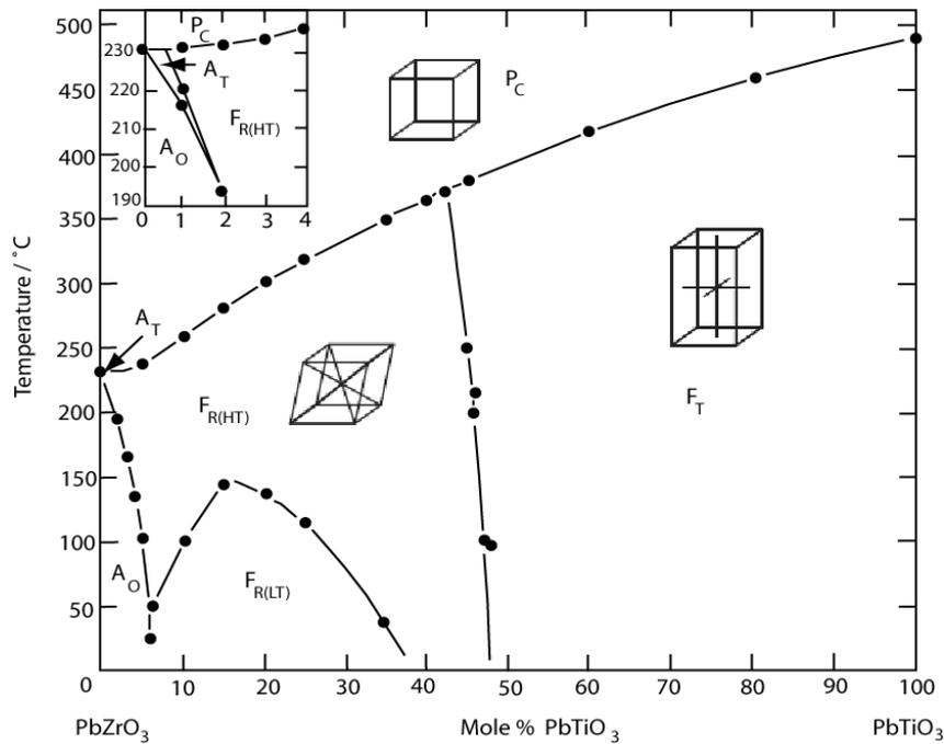
Figure 10: Phase diagram of  $\text{PbZr}_{1-x}\text{Ti}_x\text{O}_3$ , illustrating regions of phase stability for paraelectric cubic phase  $P_C$ , ferroelectric rhomboedral phases  $F_{R(HT)}$  (= high temperature) and  $F_{R(LT)}$  (= low temperature) and ferroelectric tetragonal phase  $F_T$ . From B. Jaffe, W. R. Cook, H. Jaffe, Piezoelectric Ceramics and Related Issues, Academic Press, London, 1971.
