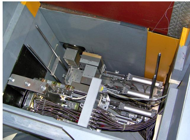
d) Shutter, filters and collimators
