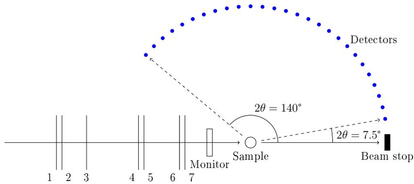
**Fig. 2:** Schematic drawing of TOFTOF. Following the neutron guide, first are choppers 1 & 2 which work together with 6 & 7 as velocity selector. Choppers 3 & 4 remove higher orders, 5 is the frame overlap chopper. The time needed for the neutrons to get from the sample to the detectors encodes their energy.
