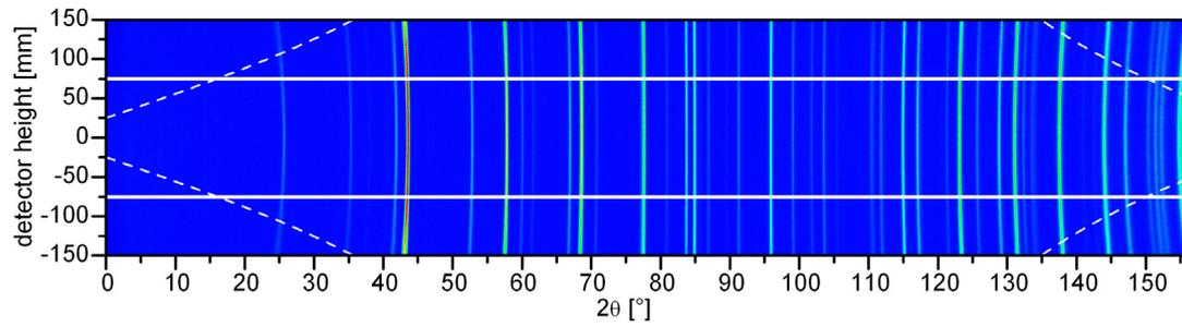
Figure 5: Two dimensional diffraction data (detector height vs. scattering angle  $2\theta$ ), collected at high-resolution powder diffractometer SPODI, illustrating the Debye-Scherrer rings of a corundum sample.
