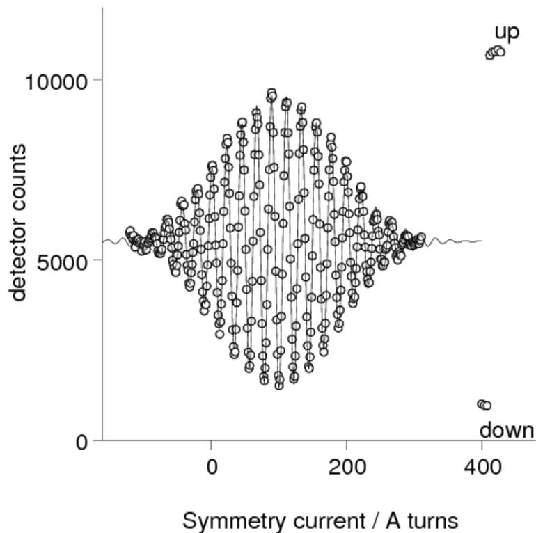
**Fig. 2:** Echo group measured with the NSE instrument.
