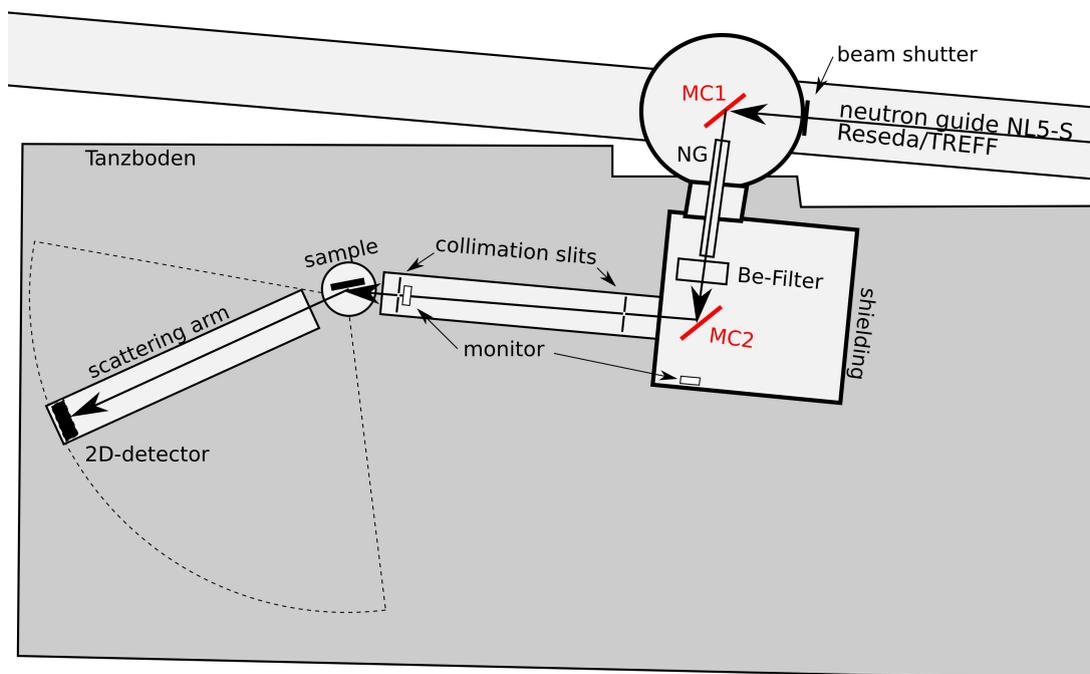
**Fig. 1:** Sketch of the reflectometer TREFF@NOSPEC in top view.
