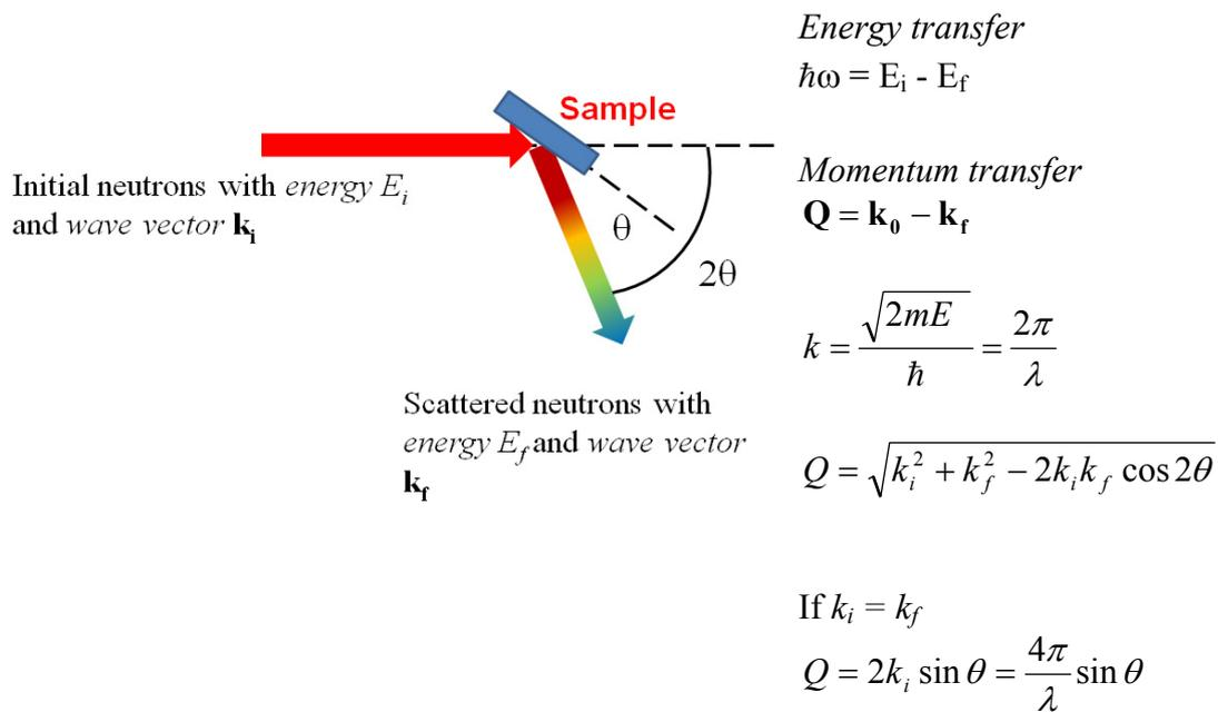
The triple axis spectrometer is designed for measuring the  $S_{coh}(\mathbf{Q}, \omega)$  in monocrystals. Therefore this function is of special interest for us.
