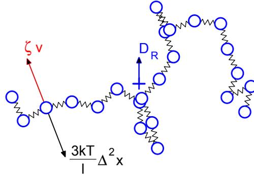
**Fig. 4:** Schematic representation of the polymer chain in the Rouse model [3] as a Gaussian chain with beads connected by springs.
