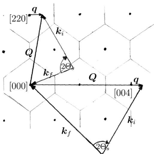
**Figure 1:** Scattering diagrams for inelastic scattering of neutrons on a fcc crystal. The reciprocal  $[1\bar{1}0]$  plane is drawn. Notation similar to the text. The energy transfer is represented by the different lengths of  $k_i$  and  $k_f$
