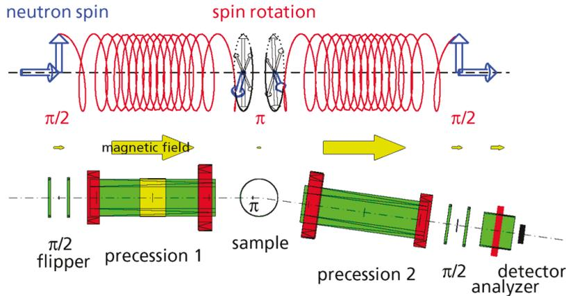
**Fig. 1:** Working principle of the NSE spectrometer [2].
