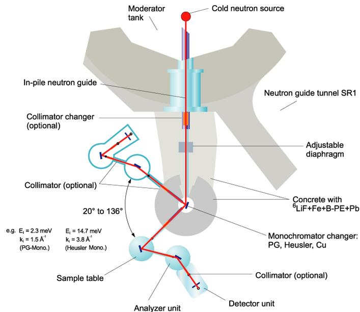
**Figure 8:** Schematic design of a three axis spectrometer.
