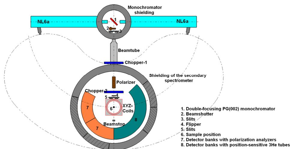
Fig. 1 The schematic layout of DNS
