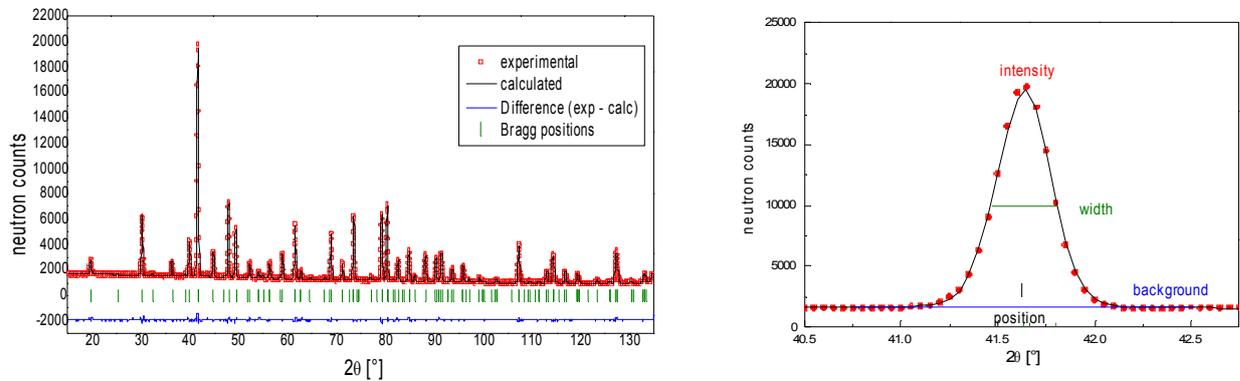
Figure 6: on the left: typical powder diffraction pattern. On the right: zoom on a single Bragg peak.
