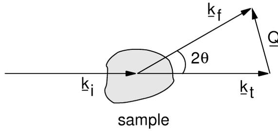
**Fig. 4:** Schematic representation of a scattering experiment.  $\mathbf{k}_{i,f,t}$  are the wave vectors of the initial (incoming), final (scattered) and transmitted neutrons, respectively.  $\mathbf{Q}$  is the scattering vector.
