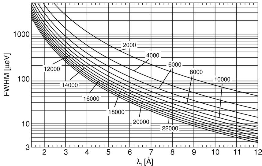
**Fig. 3:** Calculated energy resolution of the TOFTOF spectrometer shown for several chopper rotation speeds as function of the initial neutron wavelength. The chopper rotation speeds are given in rounds per minute (rpm) [4].
