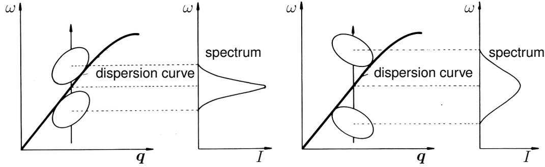
**Figure 7:** *Focused vs. unfocused measurement.*
