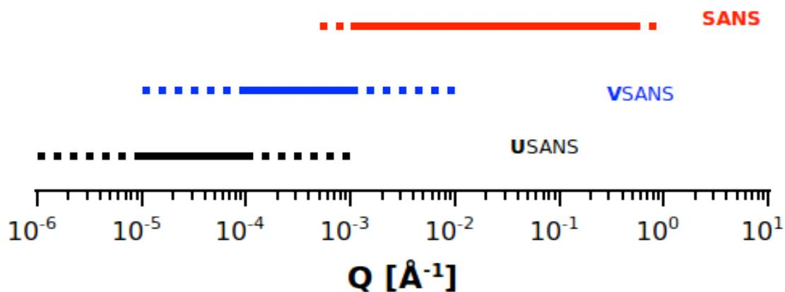
Figure 1: Focused VSANS fills space between USANS (double crystal diffractometer) and classical SANS instruments.
