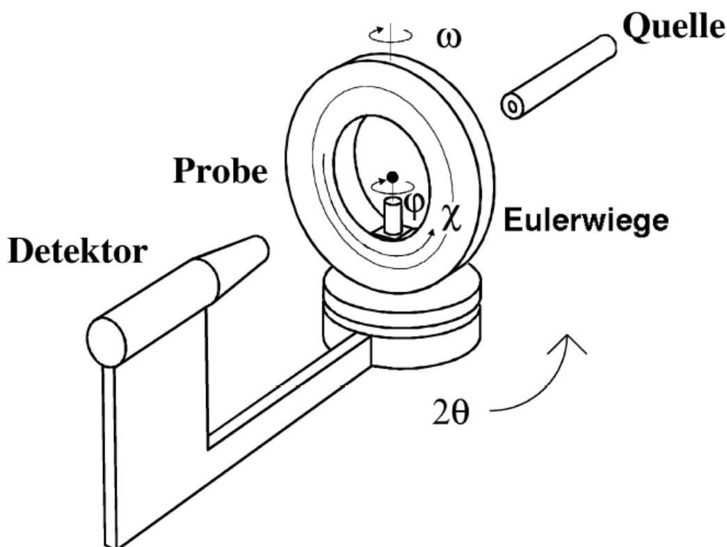
Fig. 5: Scheme of a single crystal diffractometer
