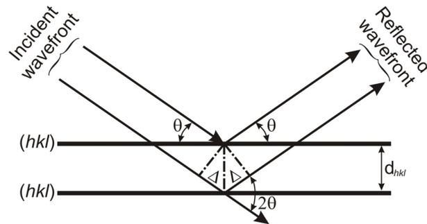
Figure 1: Illustration of Bragg's law: constructive interference of neutron waves, reflected from lattice planes, where  $\theta$ ,  $2\theta$  are Bragg angles,  $2\Delta=2d_{hkl}\sin\theta$  is the path difference and  $2\Delta=n\lambda$  is the constructive interference.
