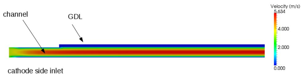
Figure 3.43: Velocity profile on the cross-sectional plane B (only the first 25 mm are showed).
