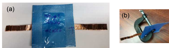
Figure 3.1: (a) Picture of a pouch bag containing a solid-state battery and (b) C-clamp improving the contact of the battery with the copper stripes.
