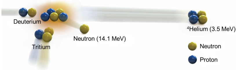
Figure 1.2: DT fusion reaction scheme [5]. D and T form an unstable ^5\text{He} nucleus, which decays with a half life time of 5.5 \times 10^{-22} s to the shown ^4\text{He} nucleus and a free neutron [6].
