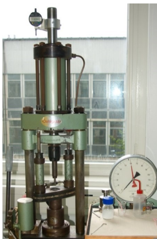
Figure 16: Hydraulic press for the fabrication of green bodies. The apparatus used here is an Oehlgass, Hahn & Kolb press.
