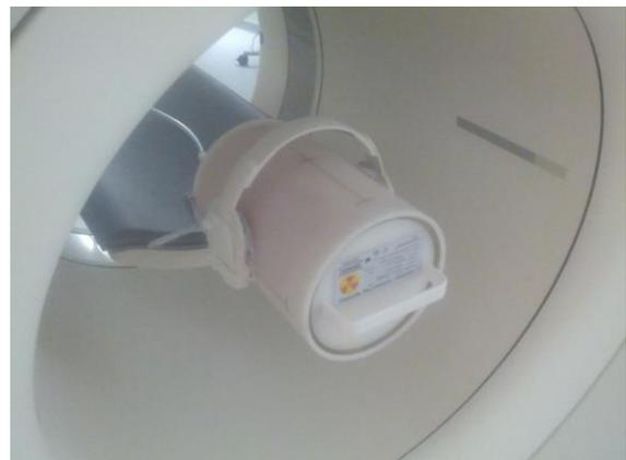
**Fig. 1:** MR-compatible headset used in this study, mounted on a PET cylinder phantom inside the Siemens mCT PET-CT scanner.
