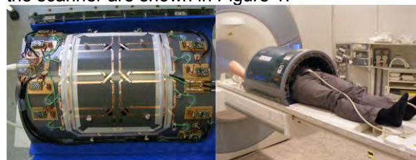
Figure 1: On the left the surface coil, on the right the coil setup inside the scanner is shown.
