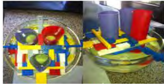
Fig. 1: Left: Photo of the phantom from top. Right: Photo from side. The interlocking plastic bricks stabilize the phantom against vibrations in the scanner.
