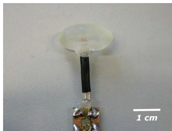
Fig. 1: Field probe, encapsulated with epoxy, susceptibility matched to the copper wire of the solenoid.
