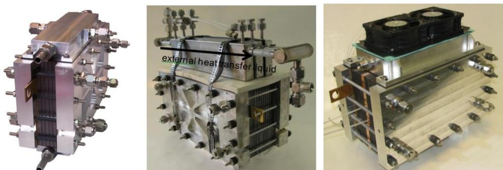
**Fig. 27: HT-PEFC stacks for the experimental analysis of cooling concepts. Left: liquid cooling after each cell. Center: heat-pipe cooling with external heat transfer to a heat transfer liquid. Right: air cooling**
