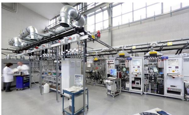
**Fig. 25:** The platform with HT-PEFC test stands which was completed in 2014
