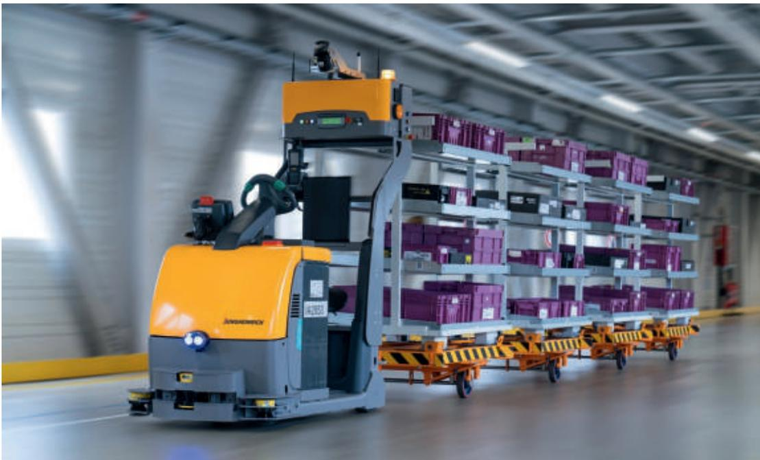
**KEEPING TRACK:** Autonomous transport, including driverless trolley trains, are already in place at a number of BMW’s plants in Germany, with plans to expand their use.
