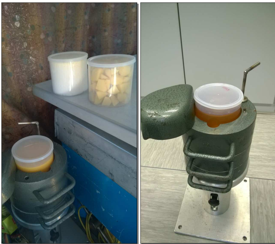
Figure 1-8: Food measuring instrument with NaI(Tl) detector and lead shielding
