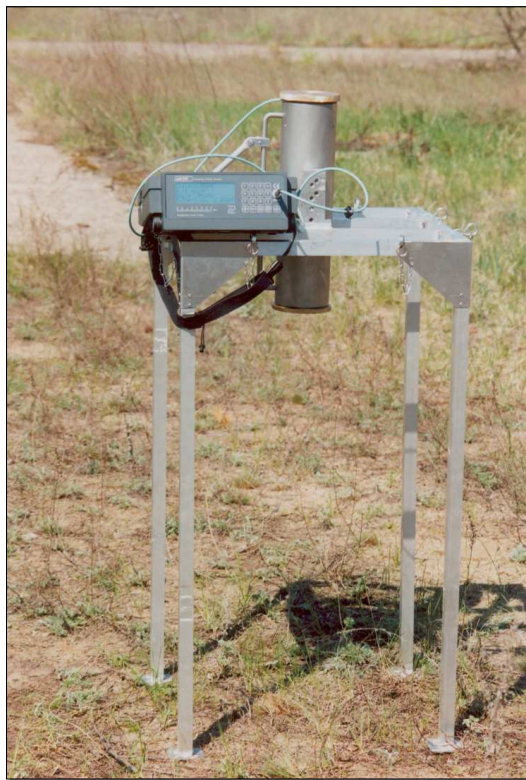
Figure 1-7: Soil measurement (local dose) with the MAB-500 measuring system
