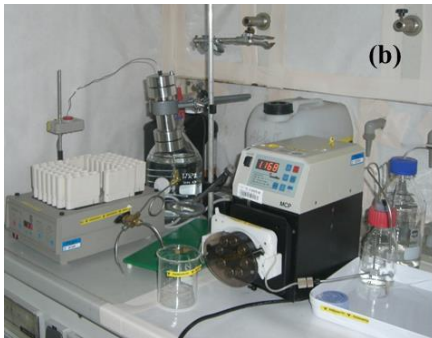
Figure 3.3 The schematic image of column setup under water saturated condition. (a) The schematic running process of column experiments. (b) The photograph of the column setup. (c) The schematic process for effluent and solid samples determination.
