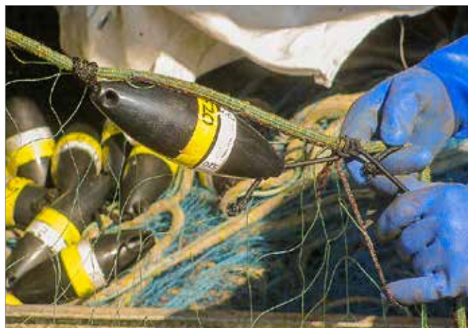
Figure 3: PALfi attached to gillnet floatline.
