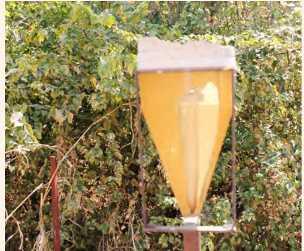
115: Pluviometric station, Chad
