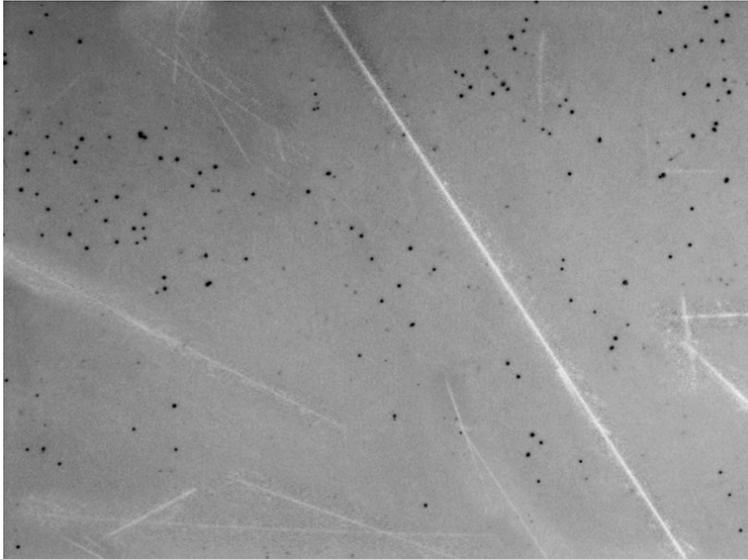
**Figure 24: Target surface after vacuum impaction, with visible score marks.**
