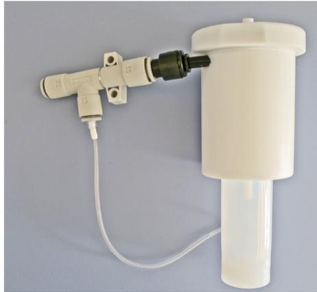
**Figure 33: Left: Schematics of Cyclone Sampler with Venturi Nozzle Inlet and right: Image of the Cyclone Sampler with Venturi Nozzle.**
