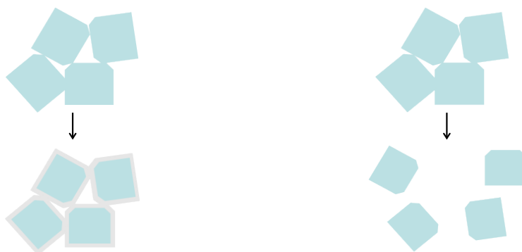
Fig. 39: Scheme of possible mechanisms for the initial incongruent dissolution: leached layer formation (left), preferential dissolution at pores and grain boundaries (right).
