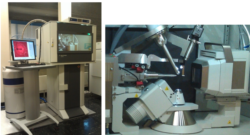
Fig. 14: Left: The complete SuperNova system. Right: The View of the SuperNova goniometer.
