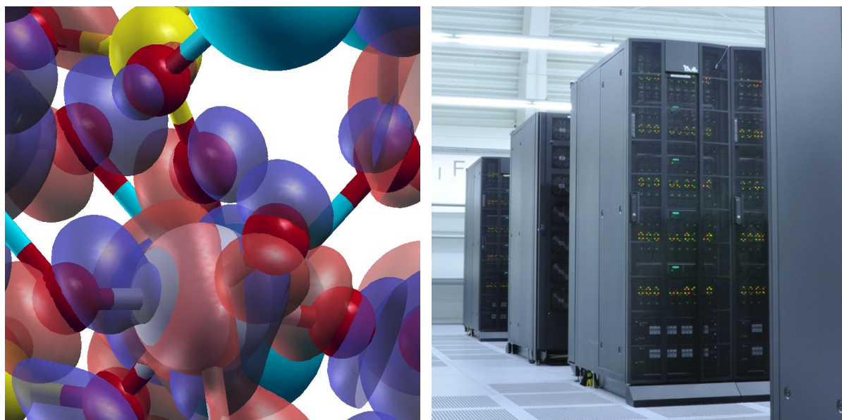
Fig. 6: Left: one of the electronic orbitals responsible for bonding between U atom (grey) and neighbouring O atoms (red) in \text{Ba}_2(\text{UO}_2)_3(\text{PO}_4)_2 borophosphate. Interaction between Uranium f orbital and Oxygen p orbitals is clearly visible. An atomic scale analysis of charge distribution provides information on the bonding environment. Right: Computer cluster at RWTH Aachen used in the investigation within Jülich-Aachen Research Alliance (JARA).
