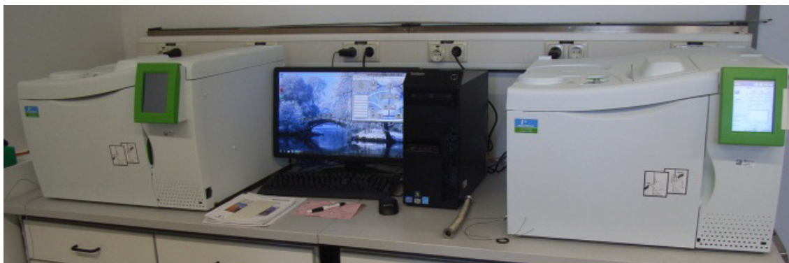
Fig. 16: Gas chromatograph PerkinElmer Clarus 580.
