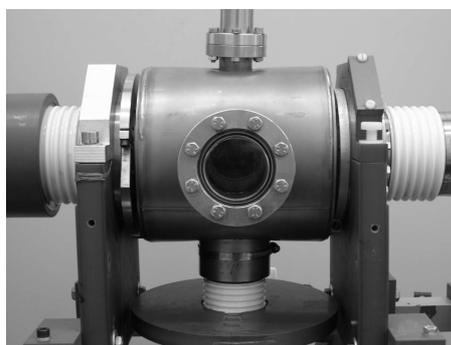
Fig. 1: High-Vacuum Set-Up with Circuit Breaker Model
