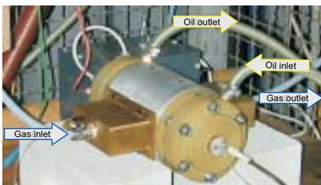
Fig. 1: Oil cooled DBD reactor
