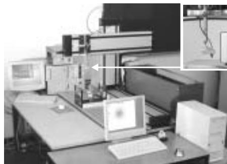
Fig. 2: Automated ultrasonic measuring setup
