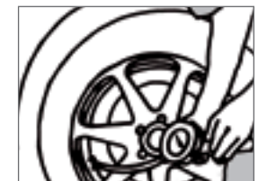
Fig. 84: Testing the air pressure
