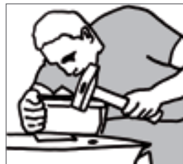
Fig.154: Bending test on the metal workpiece
