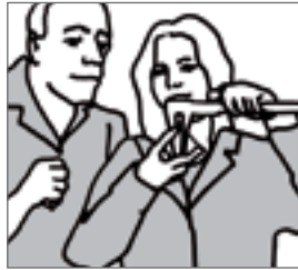
Fig. 229: Checking the accuracy of the dimensions of a work sample
