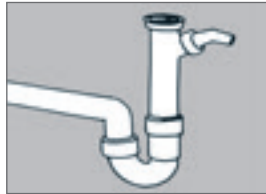
Fig. 135: Pre-assembly of the siphon
