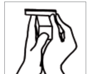
Fig. 228: Checking the surface quality by using the light-gap method
