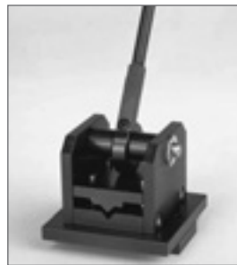
Fig. 249: The bending jig 3 shown to trainees
