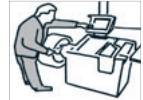
Fig. 81: Balancing the tyre with the machine
