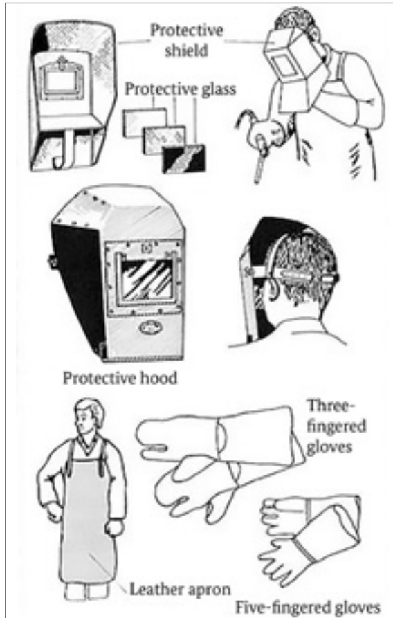
Fig. 169: Protective shield and protective clothing
