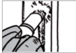
Fig. 160: Construction of a vertical seam
