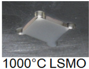
(b) STO substrate was heated several times, either in UHV or in oxygen plasma: The \text{SrTiO}_3 color changes are reversible
