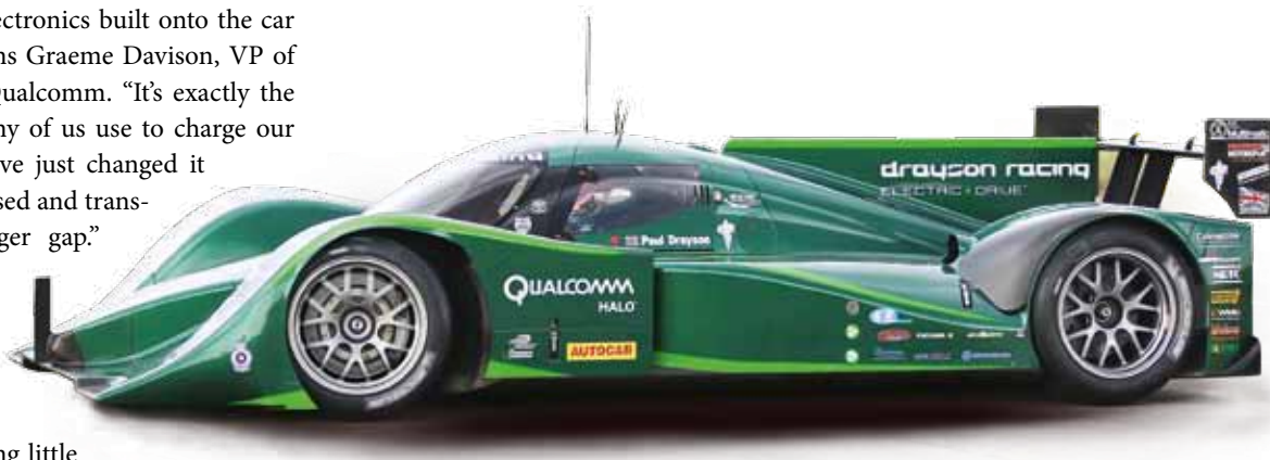
HALO EFFECT: The Halo charging system is one of the technologies showcased by the Lola Drayson B12/69 EV (above). Not a Formula E car, the vehicle was designed by Drayson Racing Technologies to become the world’s fastest electric race car. In June 2013, driven by CEO Lord Drayson, the car set a new world land-speed record for lightweight electric vehicles, hitting 204.2mph (328.6 km/h).
