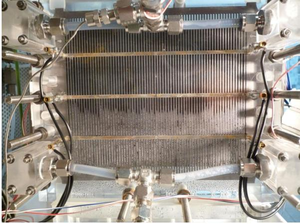
**Figure 3.3:** Image of cathode flooding in the GDL, showing distinct transition between dry, unsaturated region, and the flooded region of the cell in an experimental cell. This Plexiglas cell shows air saturated with water in the flow field, and indicates that the cathode GDL is also saturated.
