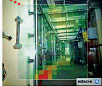
Survey on radiation source and dose rate inside the Unit 1 R/B (photo by gamma camera)
