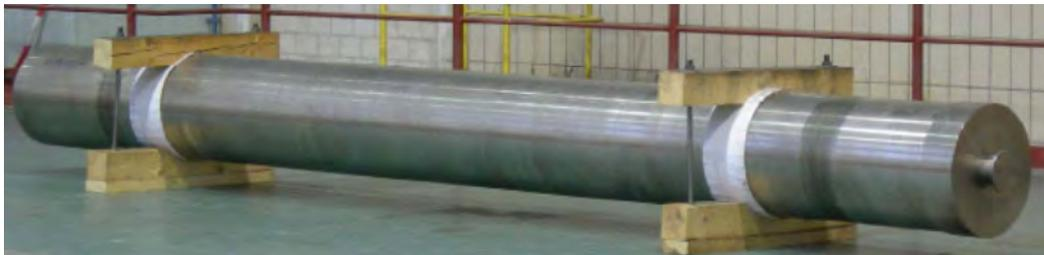
**Fig. 5.2.7** Mock-up of the BSK3 canister as used in the full-scale handling tests
