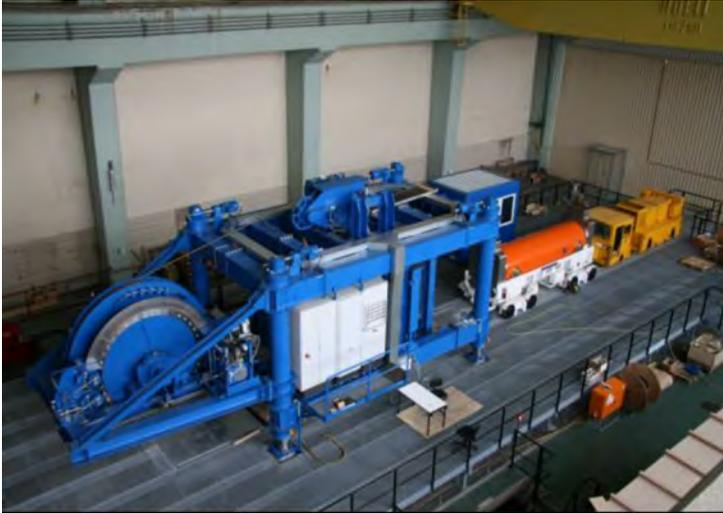
**Fig. 5.2.8** Full-scale handling test equipment for the BSK3 concept
