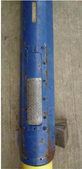
**Fig. 4.2.7** Vertical drilling system with steering ribs (Photo: Nora Röckel)
