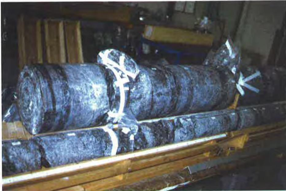
**Fig. 4.2.5** Large diameter core (245 mm) and standard core (4", 101,6 mm)
