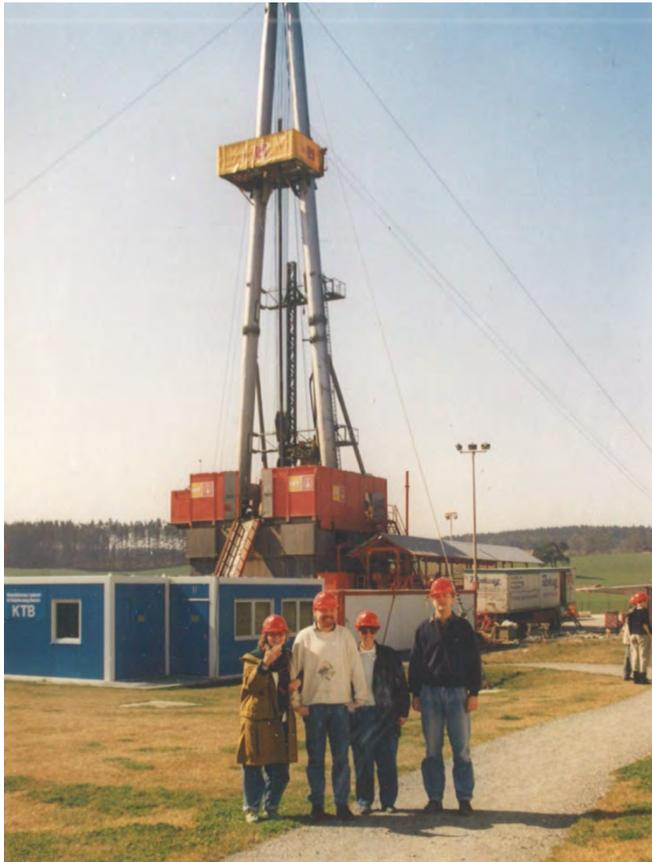
**Fig. 4.2.2** Drill rig GH 1400E for the KTB Pilot hole. Modified rotary drill rig for deep wireline coring operations
