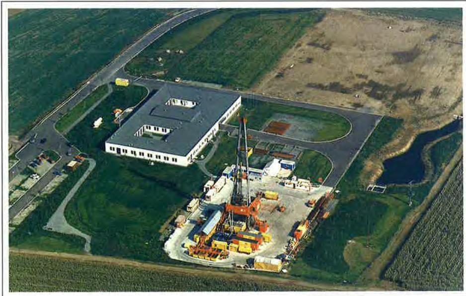
**Fig. 4.2.1** KTB Drill site. Aerial photograph with the drill rig for the KTB pilot hole in the foreground and drill site for the main hole in the background. The building on the left side is the KTB field laboratory
