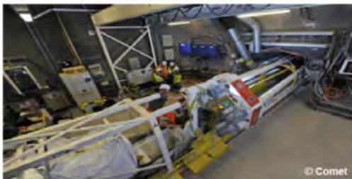
Backfilling machine passing under the gantry crane in the FE-A niche at Mont Terri
