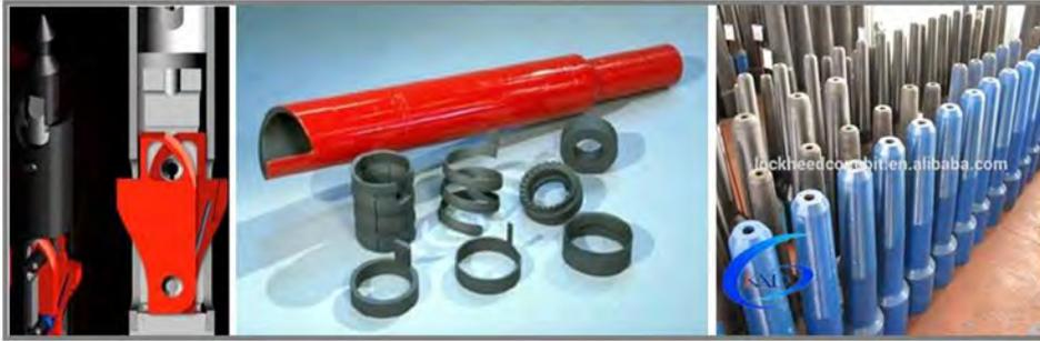
**Fig. 6.1.2** Overshot catcher with spring supported mechanical claws for deployed instrumentation in cased borehole sections (left), Overshot bell with spiral catching springs (center) and taper taps (right both for openhole fishing)
