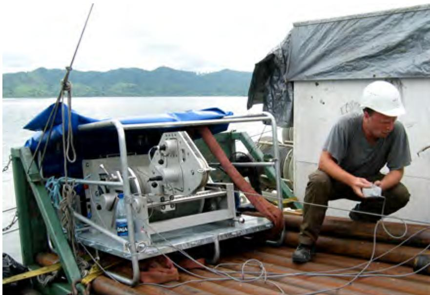
**Fig. 7.1.2** Helicopter portable logging winch with 2.2 km of a 4-conductor cable
