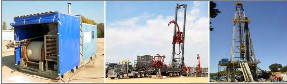
**Fig. 6.1.1** Wireline unit for logging or fishing on cable (left, a coil-tubing unit for well work-over and fishing with CT pipe (center) and a 1 million pound hook load capacity „heavy“ oilfield drill rig for drilling deep boreholes and fishing with pipe (right)
