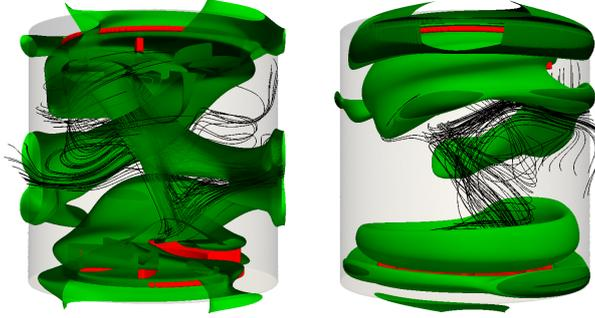
Figure 4. Isosurfaces of the mean magnetic energy  $E = 1/2\mathbf{H} \cdot \mathbf{B}$  at about 10 percent of the peak value and field lines in the saturated regime for  $Re = Rm = 506.25$  show a switch from the twisted equatorial dipole with  $m = 1$  mode at  $\mu = 1$  (left) to an axisymmetric field with  $m = 0$  mode concentrated around the impellers at  $\mu = 16$  (right).
