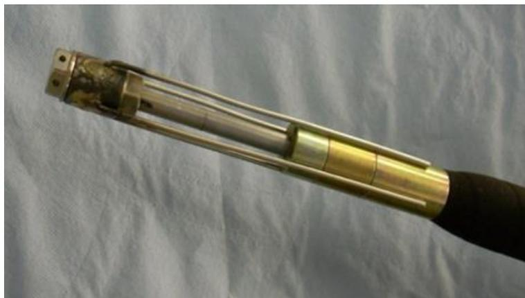
**Fig. 2.6** Sliding-end minipackers used for the PWP measurements in the long boreholes during Gallery 08 excavation
