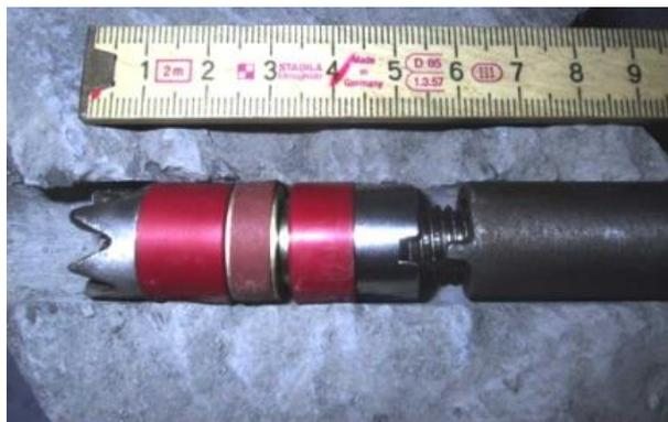
**Fig. 2.24** GRS minipiezometer for pore pressure measurement
