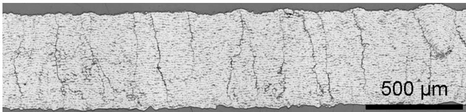
Figure 2.9: Cross section of an as-sprayed SPS YSZ free standing coating with segmentation cracks (Guignard et al. , 2012).
