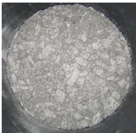
**Fig. 3.3** Photo of the crushed claystone with grains  $d < 32\text{ mm}$  after hand stamping
