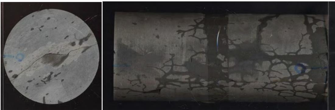
**Fig. 2.71** Micro-fissures appeared on the sample surface after heating test
