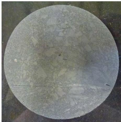
**Fig. 3.33** Inner structure of the compacted and resaturated 50 COX+50 MX80 mixture at dry density of 1.79 g/cm<sup>3</sup>
