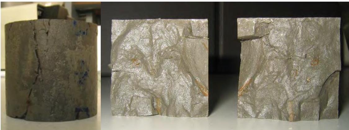
(f) COX sample EST27390B unconfined after exposing to synthetic porewater
