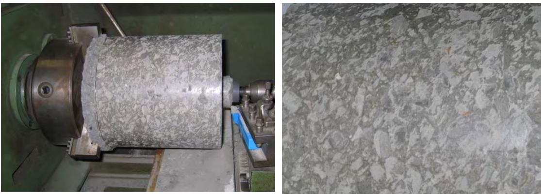
(a) Preparation of a cylinder of  $D = 250 \text{ mm}$  /  $L = 243 \text{ mm}$  from the compacted sample
