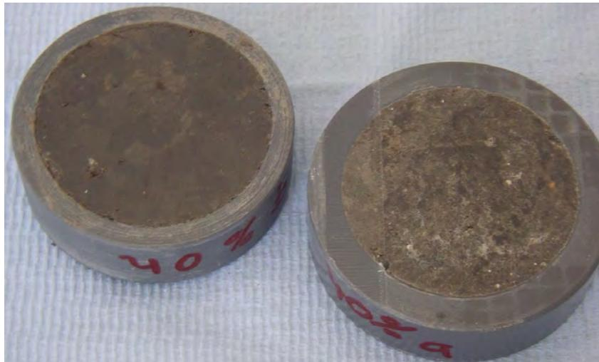
**Fig. 3.37** Photos of moulded claystone aggregate for measurements
