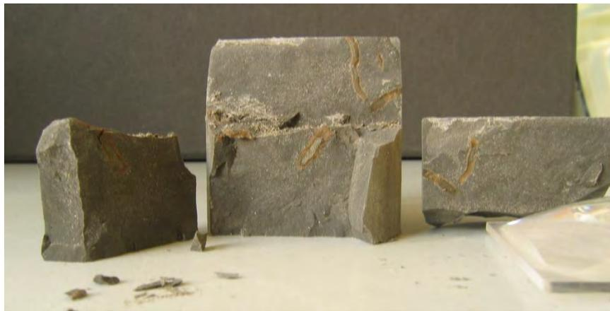
(e) COX sample EST27390A pre-confined after exposing to synthetic porewater
