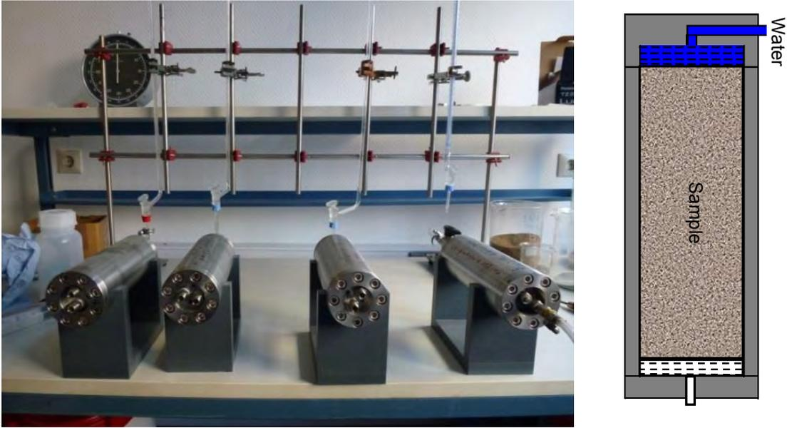
**Fig. 3.23** Test layout for saturation of compacted backfill in steel cylinder
