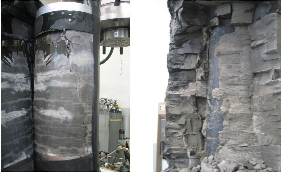
**Fig. 2.79** Pictures of the large hollow cylinder EST45592 damaged after testing
