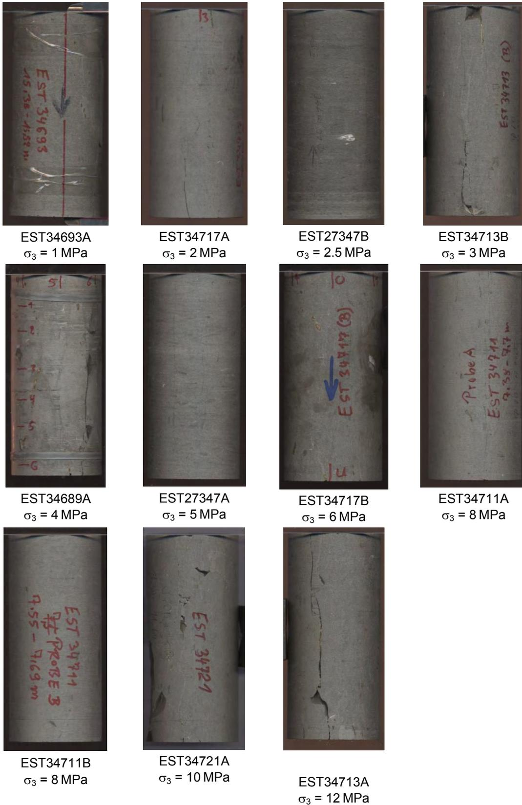
**Fig. B.10** Pictures of the first group COX samples before testing
