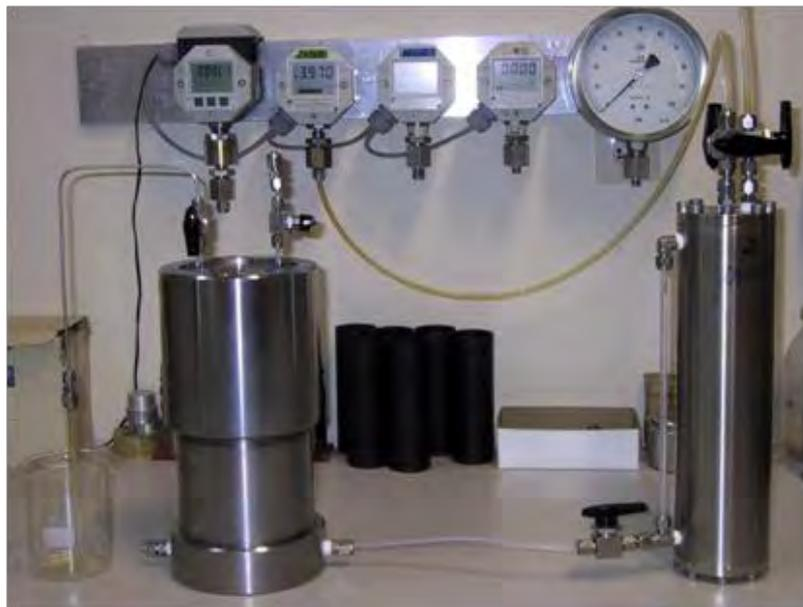
**Fig. 3.35** Test setup for measurement of water permeability of backfill materials
