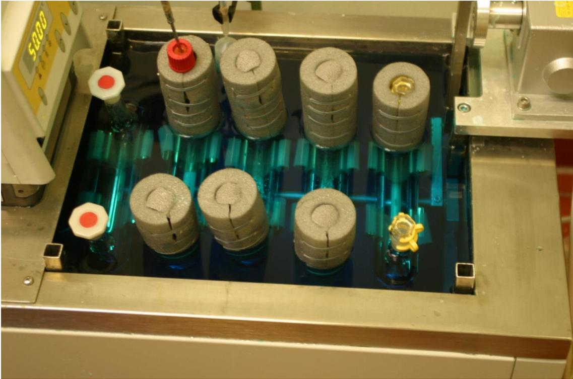
**Fig. 2.6** Glass vessel for solubility experiments immersed in an oil bath
