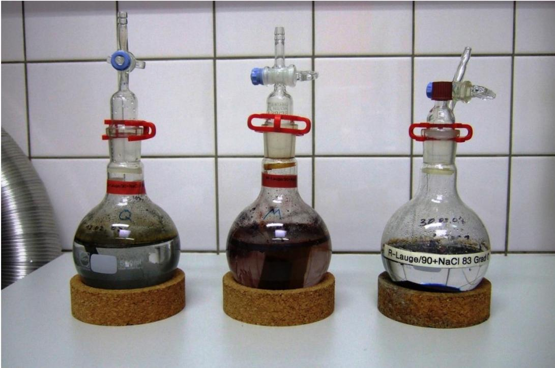
**Fig. 2.1** Round bottom flasks for the corrosion experiments
