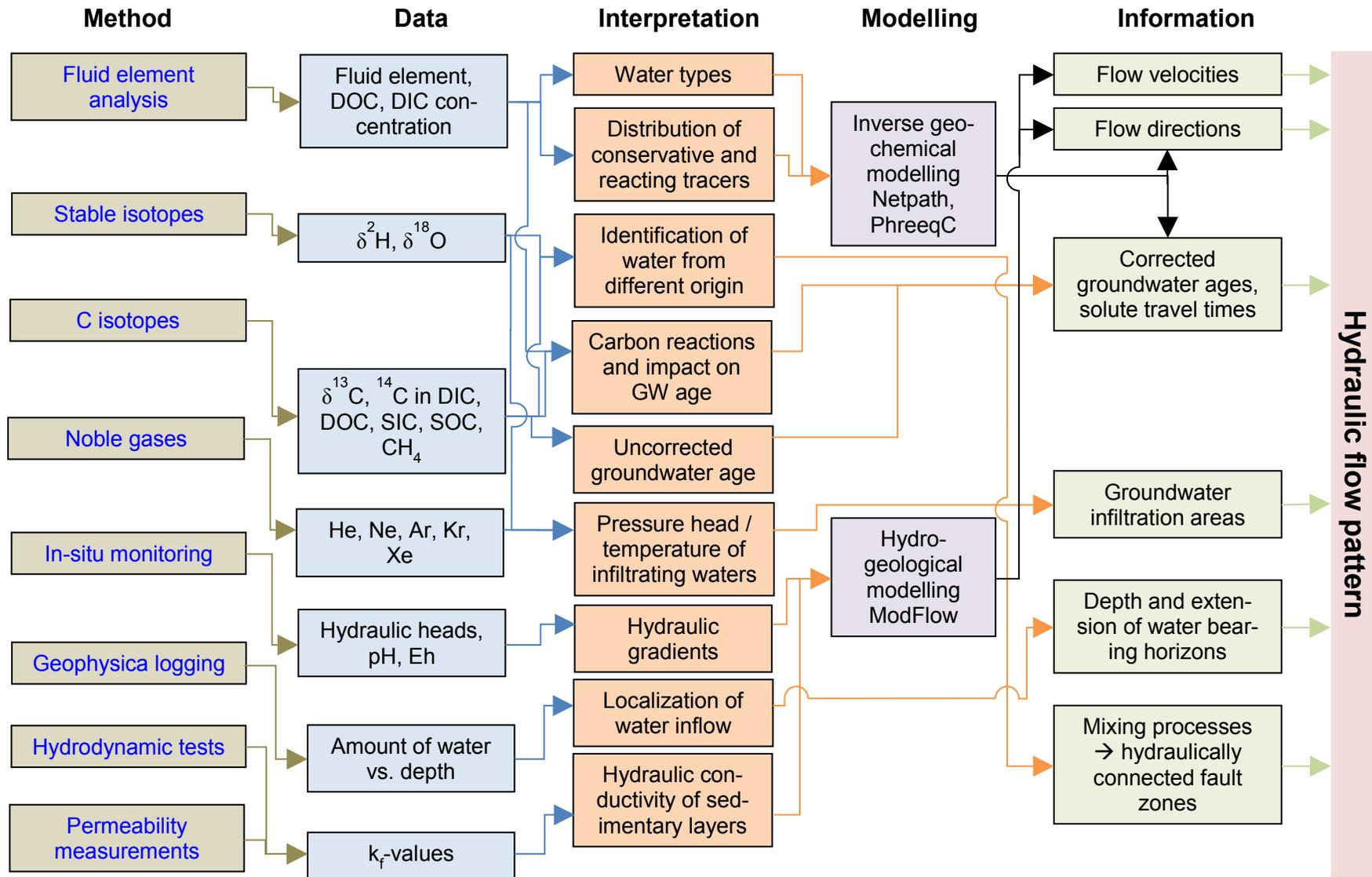
**Fig. 4.2** Evaluation scheme with methods, data, interpretation, modelling for characterization of hydraulic flow pattern
