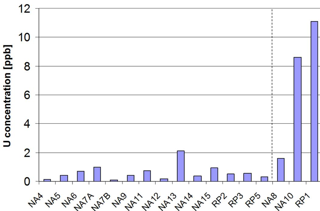
**Fig. 4.20** Uranium concentrations in the groundwater in the Ruprechtov wells. Boreholes from the infiltration area in granite: NA8, NA10, RP1
