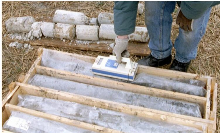
**Fig. 3.6** Identifying uranium-bearing horizons using a portable gamma ray spectrometer, applied to the drill cores
