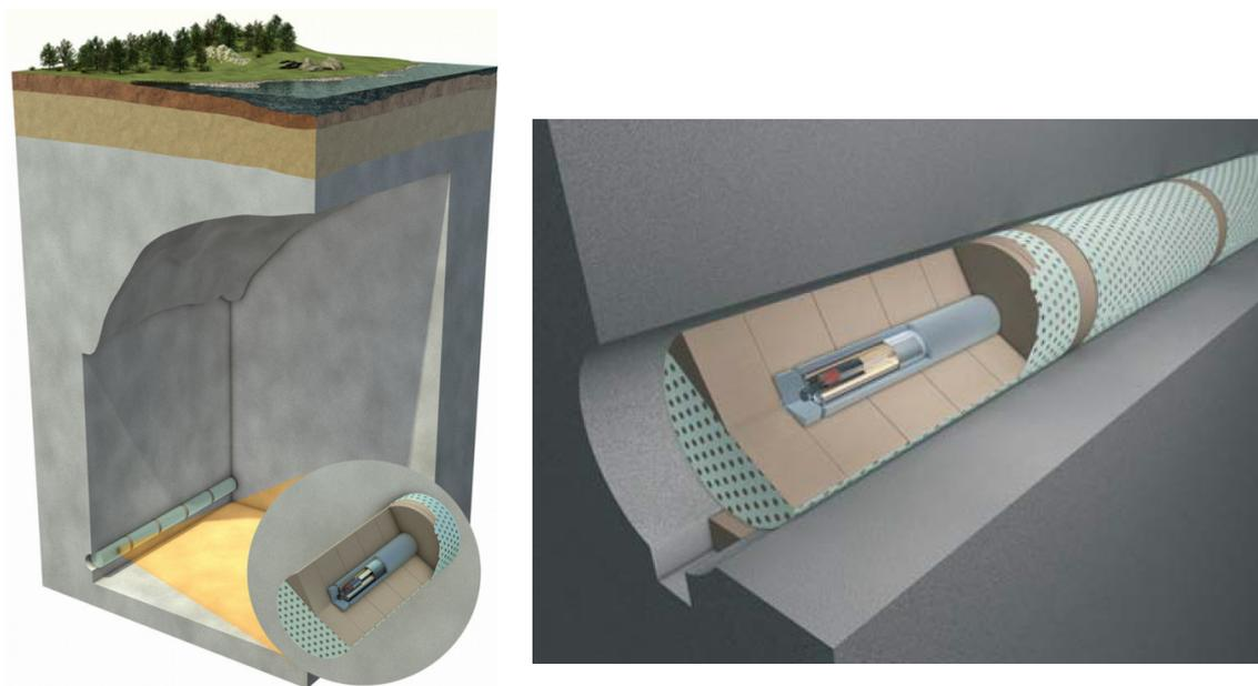
**Fig. 2.14** The schematic concept of repository system (left) and deposition hole with supercontainers (right) in the Czech Republic (SÚRAO)
