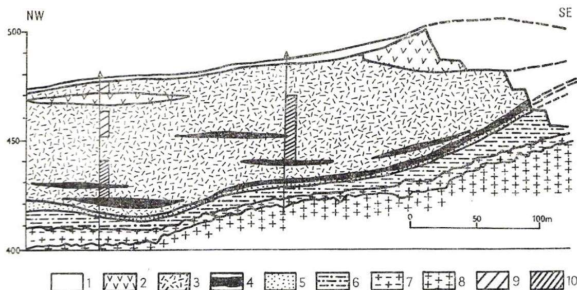
**Fig. 2.8** Schematic geological cross-section through part of the Velký Rybník bentonite deposit (close to Hájek kaolin mine)
