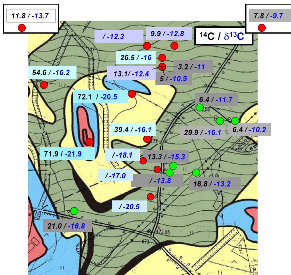
**Fig. 4.17** Distribution of <sup>14</sup>C (of DIC in pmc) and δ<sup>13</sup>C (of DIC in ‰) in different boreholes at the Ruprechtov site
