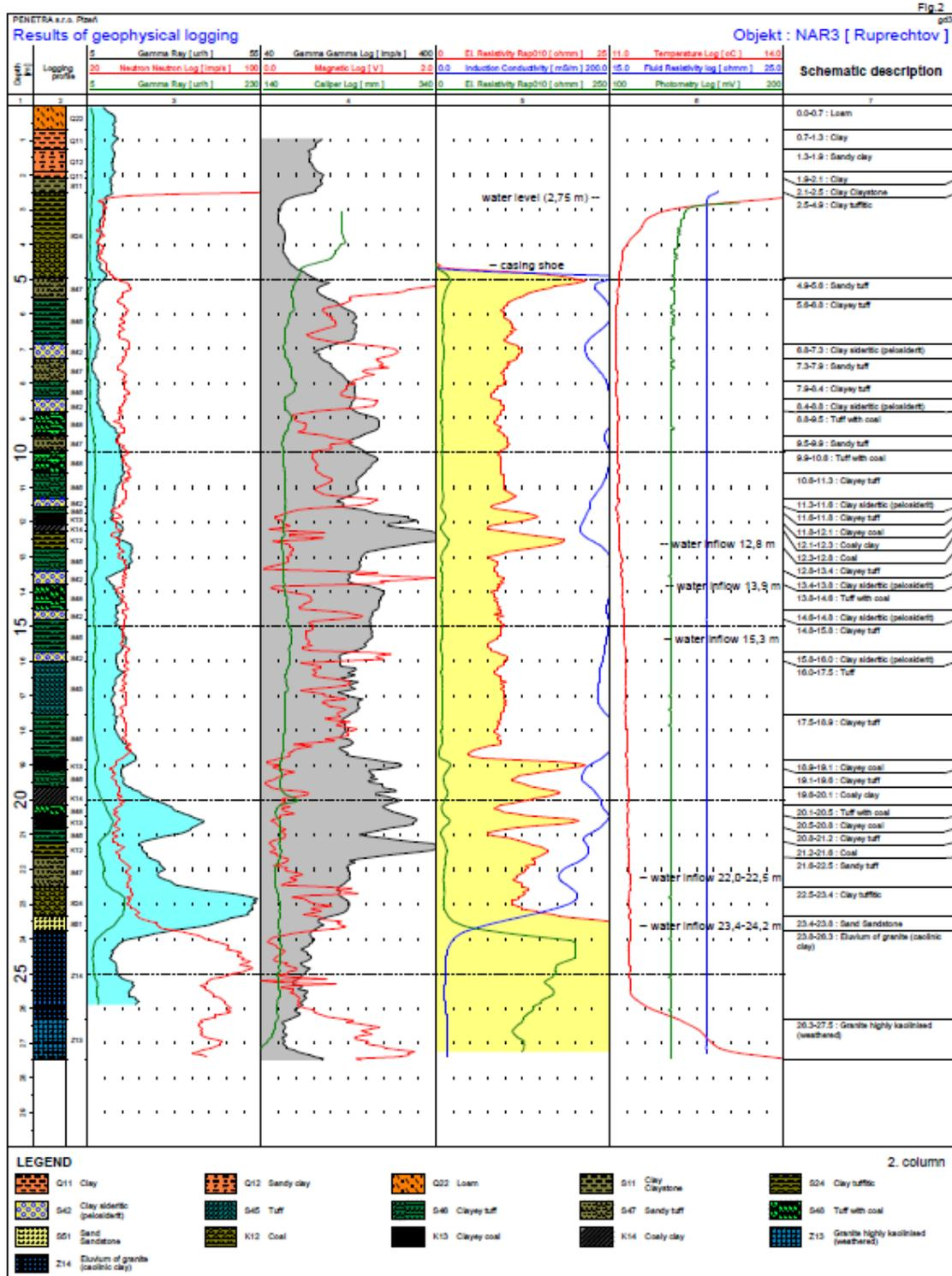
Typical output from well-logging: results from different sensors are plotted continuously against depth; in addition, e. g. the left column already represents interpretation of data (as geological profile)
