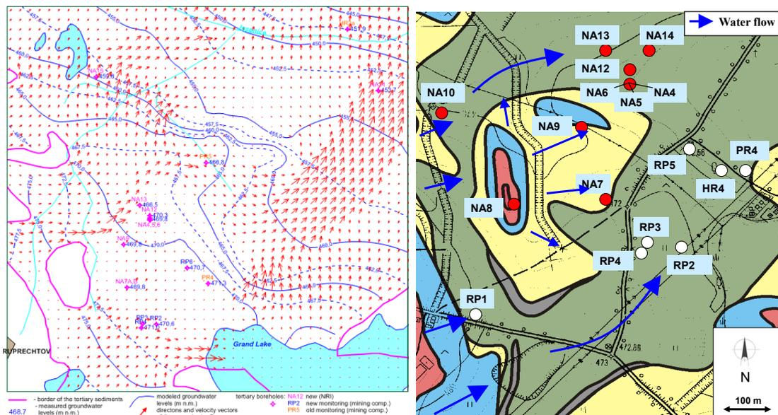
**Fig. 4.6** Results from the flow modelling and conceptual model of groundwater flow pattern in the Tertiary basin of the studied Ruprechtov aquifer system
