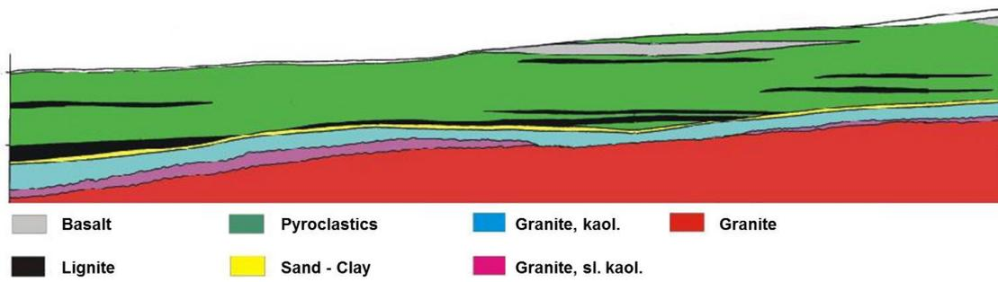
**Fig. 1.3** Schematic geological cross-section of Hájek South deposit (from /NOS 02/, modified after unpublished ÚJV-documents)
