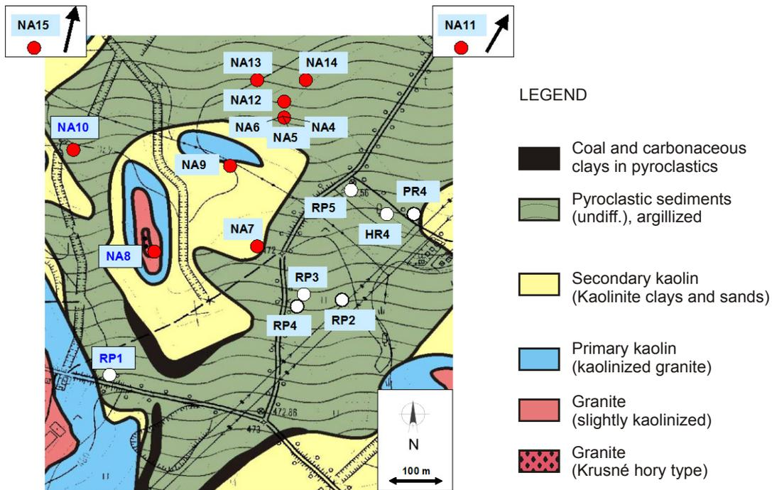
**Fig. 4.1** The location of boreholes at the Ruprechtov site, shown on the background of the geological map
