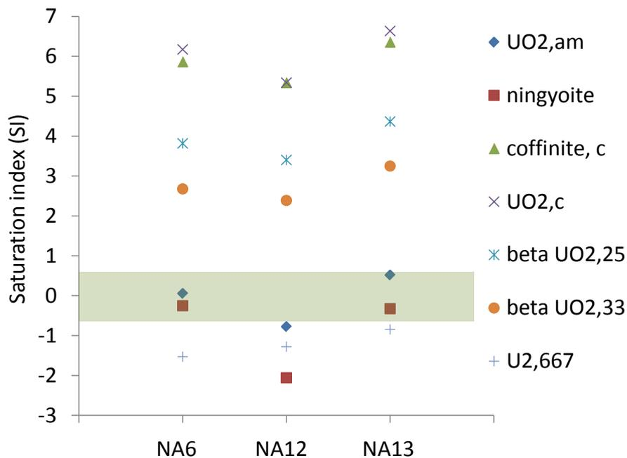
**Fig. 4.23** Saturation indices of various U(IV) minerals calculated for groundwaters NA6, NA12 and NA13
