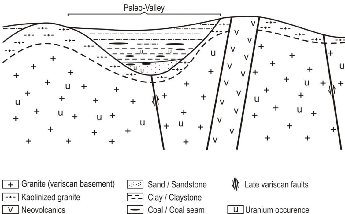
**Fig. 2.4** Schematic cross-section showing the main geological features of the Ruprechtov area including the occurrence of uranium in granite (broadly disseminated) and in Tertiary sediments (locally accumulated in layers)
