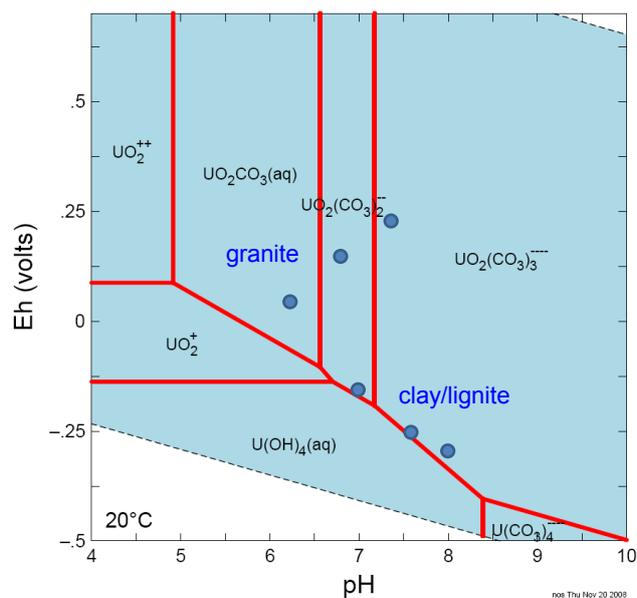
**Fig. 4.21** pH/Eh diagram for Ruprechtov groundwater; U concentration  $10^{-3}$  mg/L,  $\text{CO}_2$  activity =  $10^{-3}$
