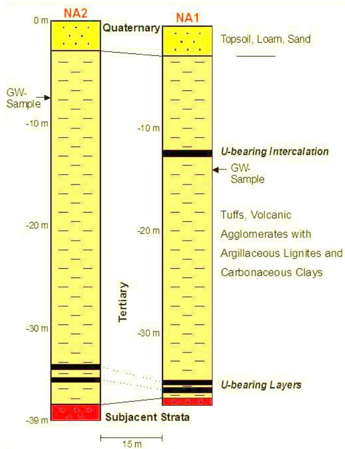
**Fig. 2.11** Basic results from first core drills NA1 and NA2, verifying main U-accumulation in the lowermost part of the Tertiary (volcano-detrital) formation (“U-bearing layers”) (from /BRA 98/, slightly modified)
