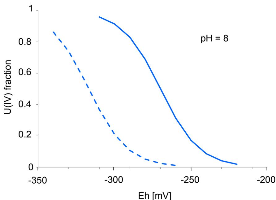
**Fig. 4.22** Fraction of U(IV) in dependence of Eh-value at pH 8, for conditions of NA6 groundwater for calculations without (bold line) and with consideration of  $(\text{Me}^{2+})_n\text{UO}_2(\text{CO}_3)^{-(4-2n)}$  complexes (dotted line)
