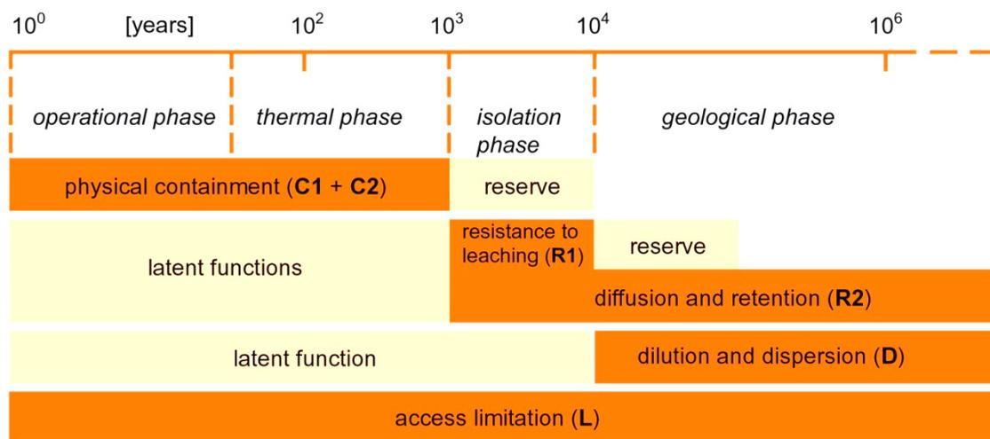
**Fig. 1.1** The four phases in the normal evolution of a deep disposal system for the vitrified waste and spent fuel, and the corresponding long-term safety functions /OND 01/
