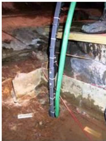
**Fig. 5.15** Insertion of an electrode chain into a measuring borehole in the rock between deposition hole #5 and #6 in Section II
