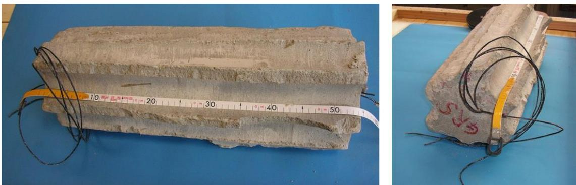
**Fig. 8.2** Core section from the top central buffer of deposition hole #5 with embedded electrode chain
