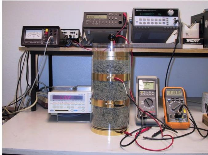
**Fig. 4.5** Measurement set-up for determination of backfill resistivity
