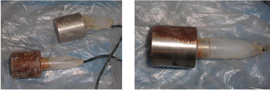
**Fig. 8.1** Electrodes from the backfill in Section II showing surface corrosion
