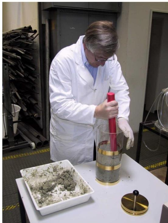
**Fig. 4.4** Emplacement of moisturized backfill into measurement cell for determination of material resistivity
