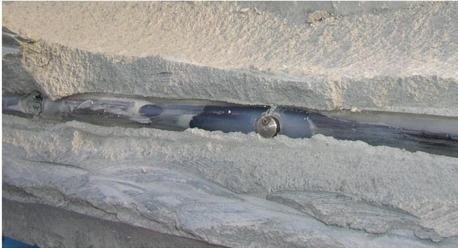
**Fig. 8.3** Electrode chain embedded in the buffer
