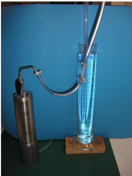
Fig. 3.23 System for measurement of sand/bentonite permeability to gas (left) and water (right)
