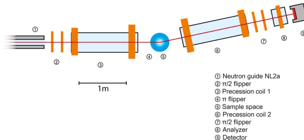
Figure 2: Schematic drawing of J-NSE set-up, top view.
