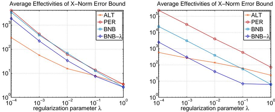
Fig. 5.5: Average  $X$ -norm error bound effectivities (over  $M$  and  $\Xi_{\text{test}}$ ) vs. regularization parameter  $\lambda$  for Graetz flow (left) and heat transfer problem (right)
