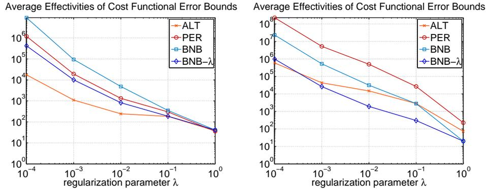
Fig. 5.6: Average cost functional error bound effectivities (over  $M$  and  $\Xi_{\text{test}}$ ) vs. regularization parameter  $\lambda$  for Graetz flow (left) and heat transfer problem (right)
