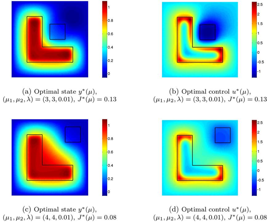
Fig. 5.3: Optimal state  $y^*(\mu)$ , optimal control  $u^*(\mu)$ , and optimal cost functional value  $J^*(\mu)$  for different representative parameter values
