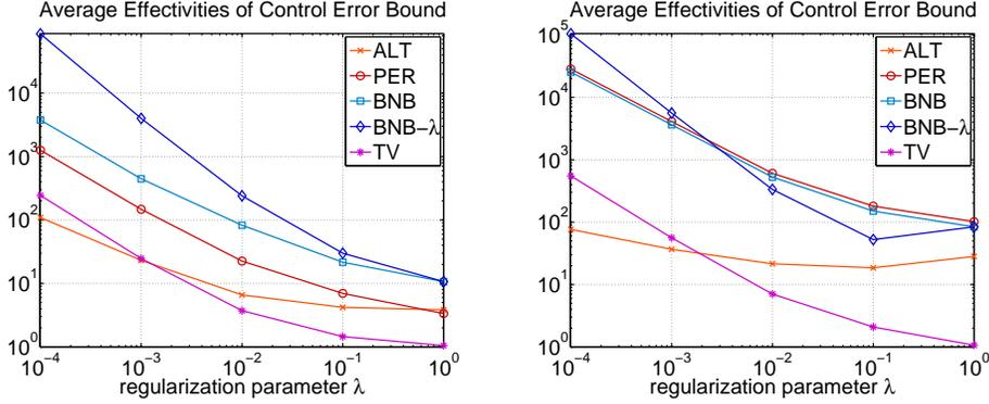
Fig. 5.4: Average control error bound effectivities (over  $M$  and  $\Xi_{\text{test}}$ ) vs. regularization parameter  $\lambda$  for Graetz flow (left) and heat transfer problem (right)
