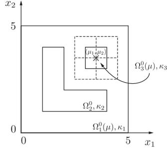
Fig. 5.2: Parametrized domain  $\Omega^o$  for the heat transfer problem with distributed control.
