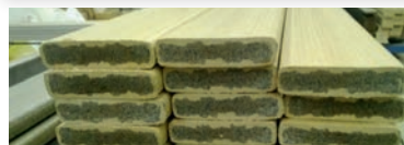
Multilayer WPC-decking boards with recycled ABS(45%) +wood (55%) inside and recycled PE or PP (35%) +wood (65%) outside
