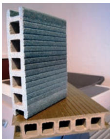
Multilayer WPC-decking boards with recycled ABS(45%) +wood (55%) inside and recycled PE or PP (35%) +wood (65%) outside
