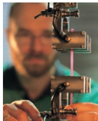
Testing mechanical properties of biobased plastics
