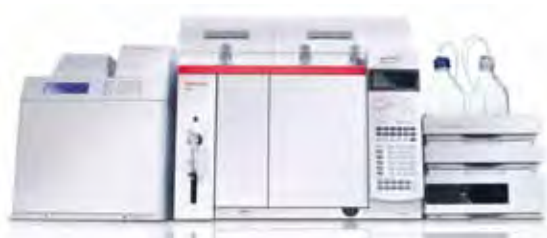
High Temperature Size-Exclusion Chromatography (picture: Polymer Charr).
