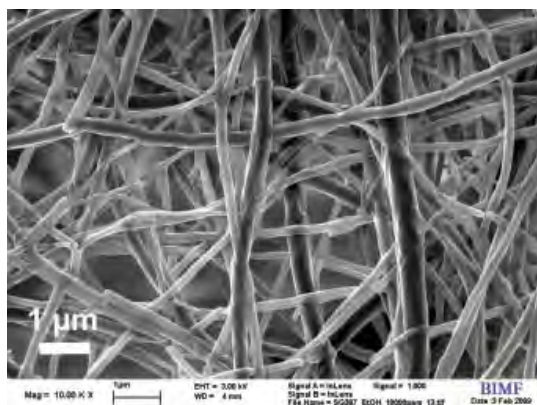
Fig. 1: Nonwoven from PP fibres with integrated nanofibres from benzene-1,3,5-trisamides (MC I, Bayreuth)
