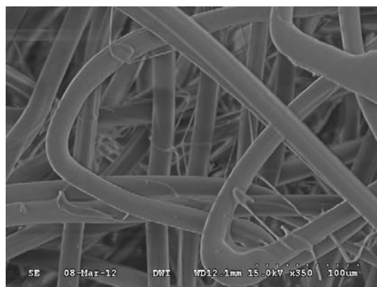
Fig. 2: Nanofibre-bearing PP-felt after application of commercially available hydrogelators on basis of polyurethane/urea
