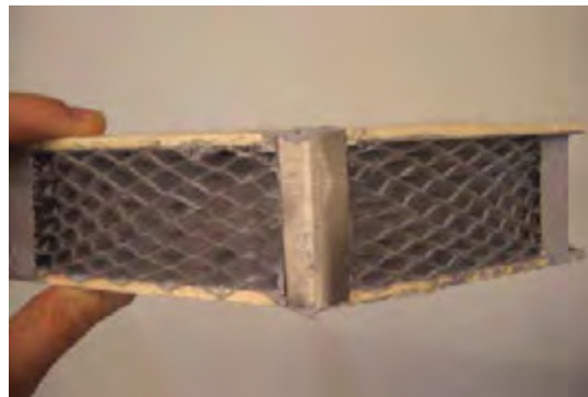
Figure 2: Prototype of a membrane module for air conditioning systems (Foto: AVT RWTH Aachen University)
