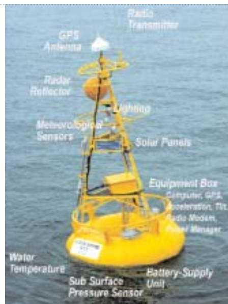
Set-up of the GPS-equipped buoys to be installed in Indonesia in November 2005 Source: BMBF
